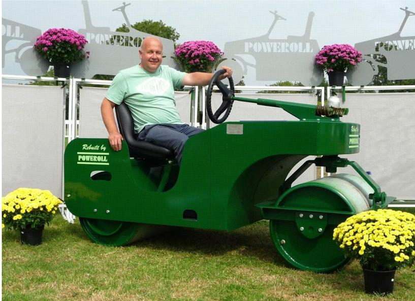
We completely rebuild old Auto-Roller AR3's. The original engine, gearbox and clutch are discarded in favour of a new user friendly Poweroll built hydraulic drive kit. All other components are replaced as wear on the original requires.
