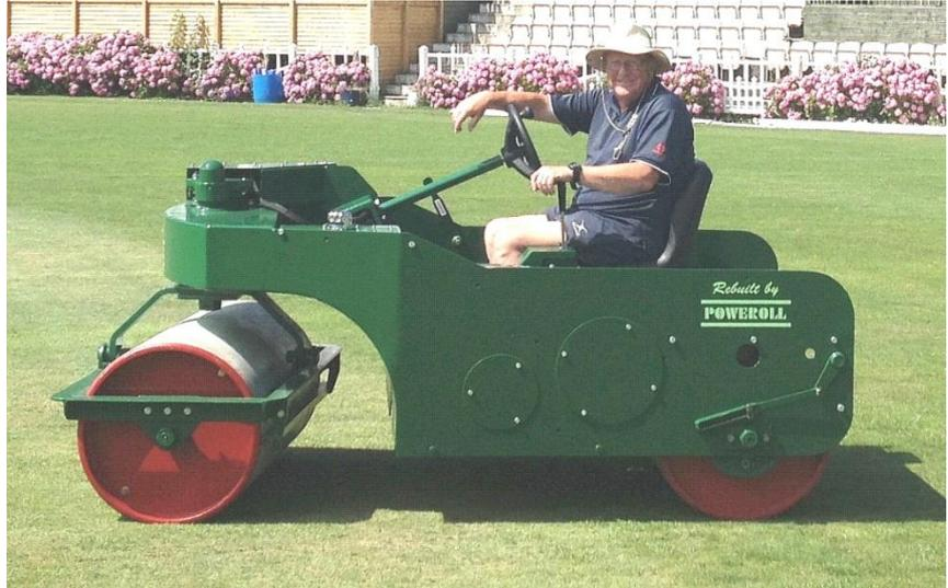
They are very basic machines, having minimal options to vary the ballast, in fact just the roller drums.
