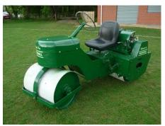
Left, Upgrade kit fitted to a Greens Griffin roller. A little more work requiring an angle grinder is required to remove the original brackets in the engine bay, to fit the kit to this roller. But the excellent results more than justify the effort required.
